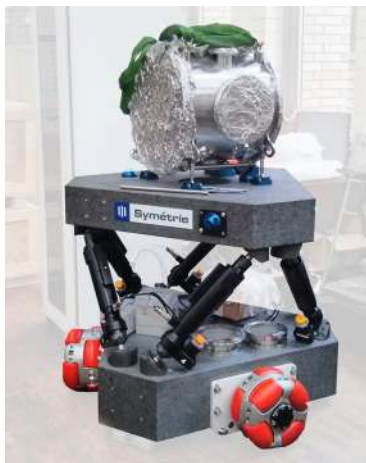
JORAN hexapod size has been adapted to the beam height of the Australian Synchrotron.
