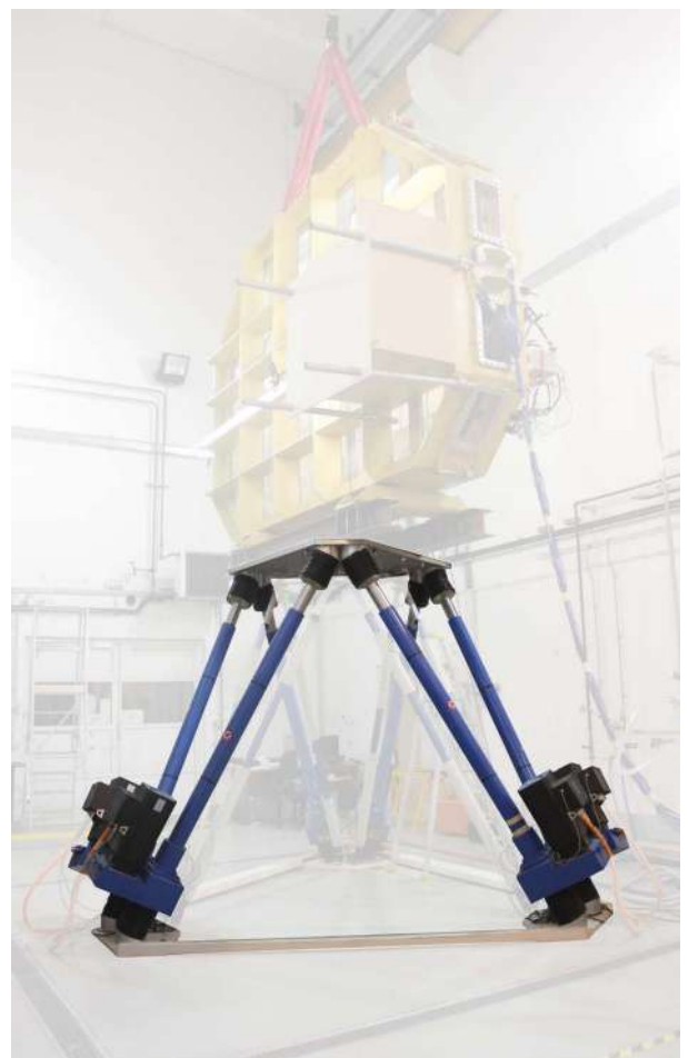
Sloshing tests hexapod AQUILON with a 10T payload.
