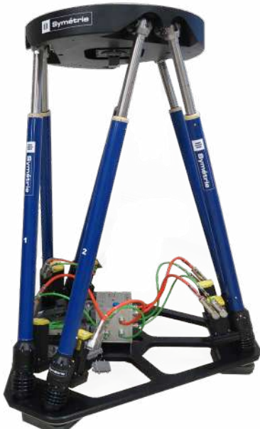
This customized hexapod with extra travel range enables the qualification of space optical instruments. Hexapod height in middle position: 1400 mm / Payload: 200 kg.
