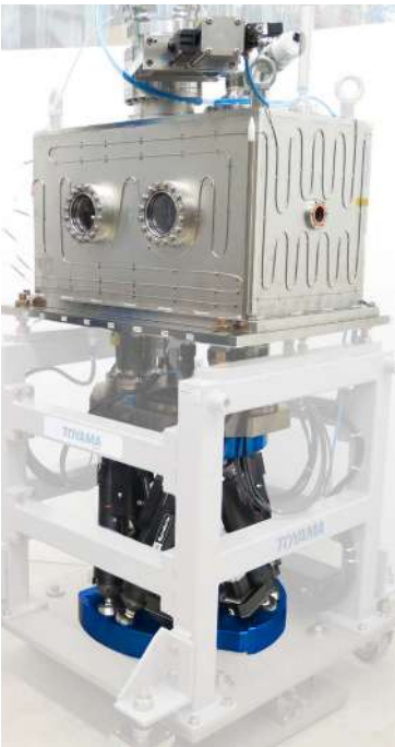
KUBAN hexapod aligns a polarimeter with high precision in a short time. This installation made by TOYAMA can be moved to be used on different beamlines at MAX IV Laboratory synchrotron.
