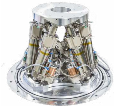
Custom ZONDA hexapod for 10^{-3} mbar vacuum
