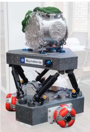
JORAN hexapod size has been adapted to the beam height of the Australian Synchrotron.
