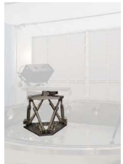
A vacuum compatible ZONDA hexapod is used at CSL to calibrate space optical instruments.
