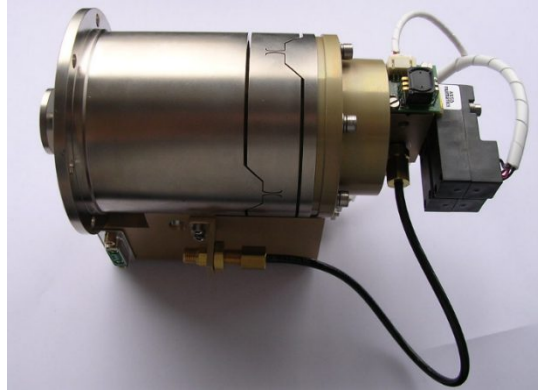
Figure 2. Axial actuator: schematics and picture of hardware
