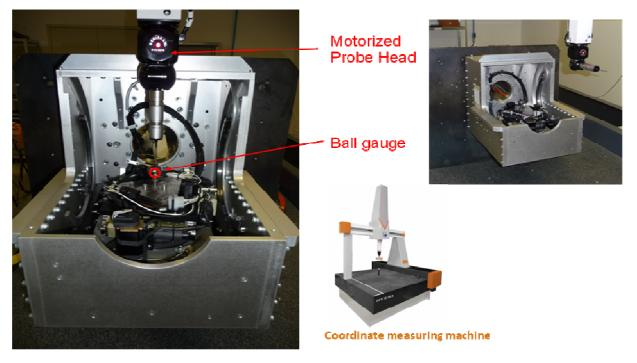
Figure 3: Goniometer on the coordinate measuring machine
