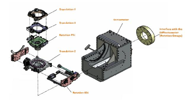
Figure 2: Exploded view of the goniometer
