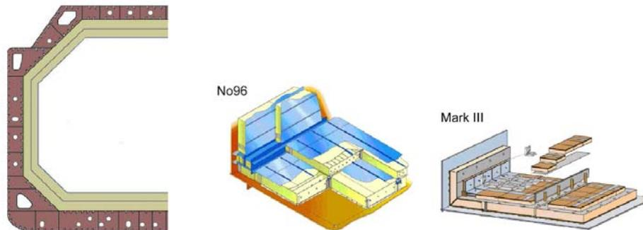
Figure 1 Membrane type LNG tank and different containment systems
