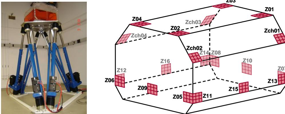
Figure 3 Small scale sloshing model tests (GTT) using hexapod and typical pressure sensors positions
