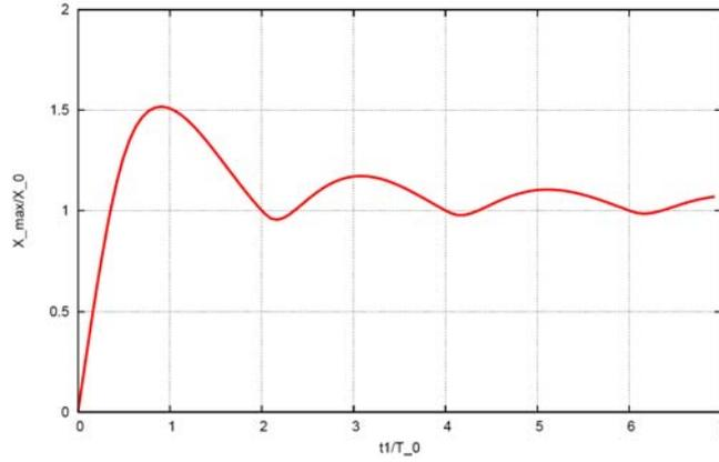
Figure 12 *Dynamic amplification factor for triangular impulsive loading ( $t_1$  impulse duration,  $T_0$  – natural period of the dynamic system). The loading is symmetrical around  $t = t_1/2$  where it takes the maximum value  $F_0 = kx_0$*
