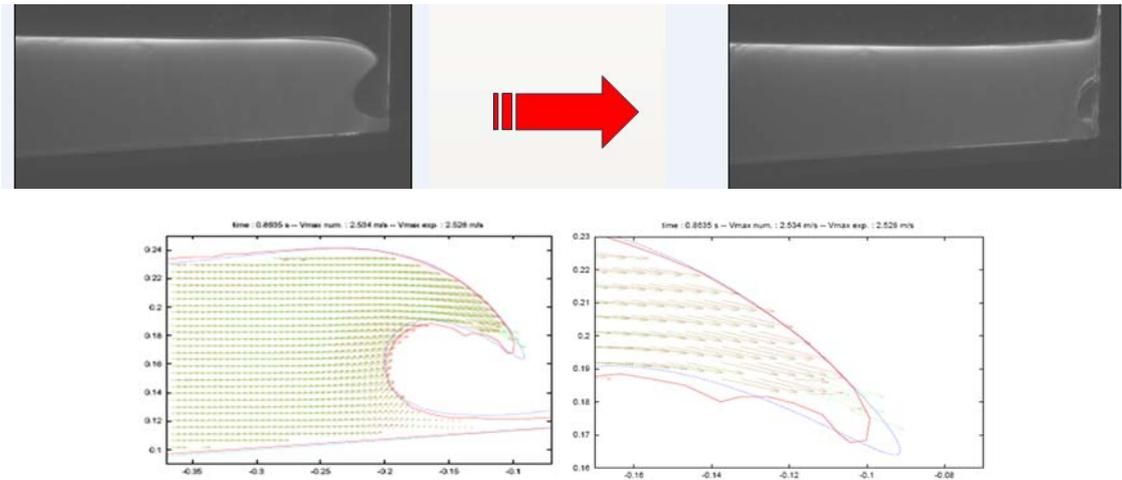
Figure 5 Hydroelastic impact tests in the wave flume at moderate scale and numerical simulations of the wave kinematics before impact
