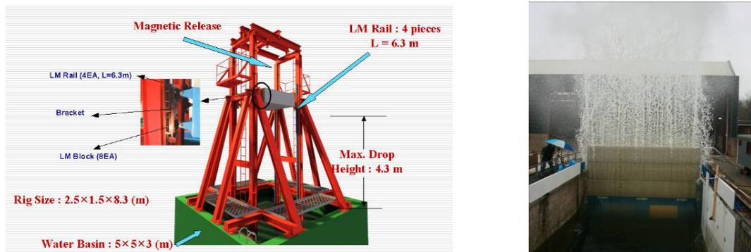
Figure 4 Full scale impact tests (left – drop tests, right – impacts in wave flume – *Sloshel* project)
