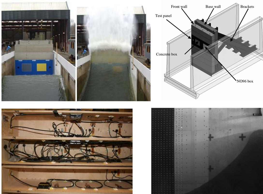
Figure 6 *Sloshel* model tests (clockwise: wave flume, mounting scheme, iCAM sensor and instrumented NO96 box)
