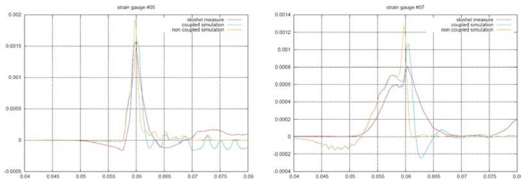
Figure 15 Comparison of calculated and measured strains at strain gauges #5 (left) and #7 (right) for a flip through impact.
