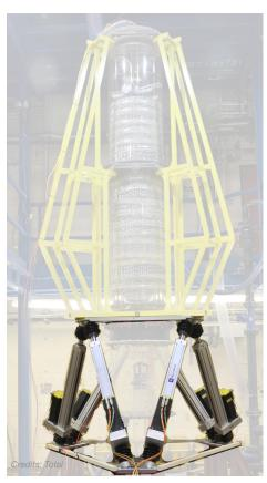
MISTRAL hexapod simulates the motion of a floating gas production unit to characterize hydrodynamic effects of the swell on the chemical reactions in a gas deacidification column. These tests allow to improve performance and robustness of the processing units.
