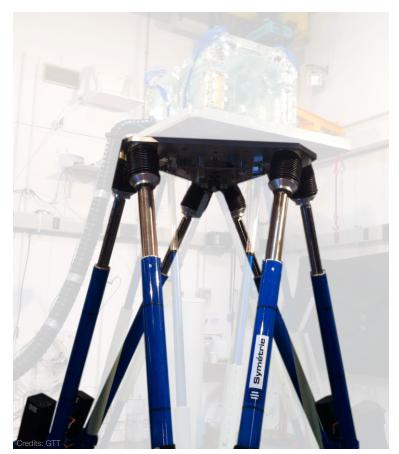
GTT designs cryogenic membrane containment systems used in the shipbuilding industry for the transport of liquid natural gas (LNG). SIROCCO hexapod allows GTT laboratories to study the impact of moving liquid, also called sloshing, on their insulation.
