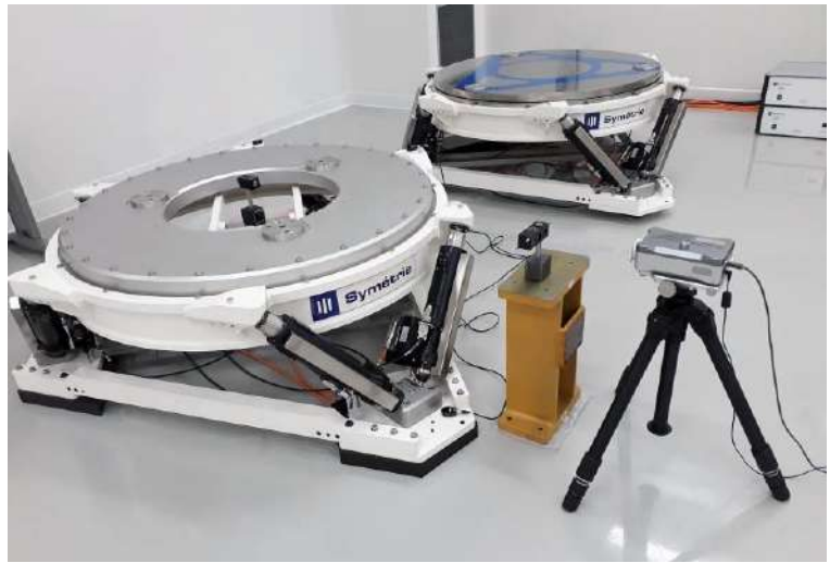
CREDITS: SYMETRIE - HEXAPODS USED TO POSITION THE SEGMENTS AND THE REFERENCE
