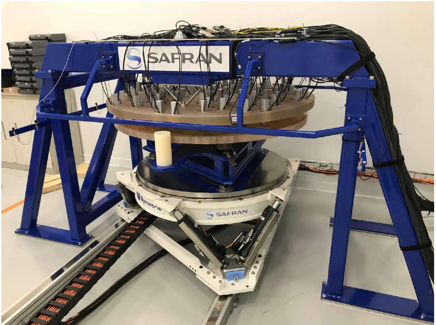
CREDITS: SYMETRIE - HEXAPOD CHARACTERIZING THE MIRROR BLANK
