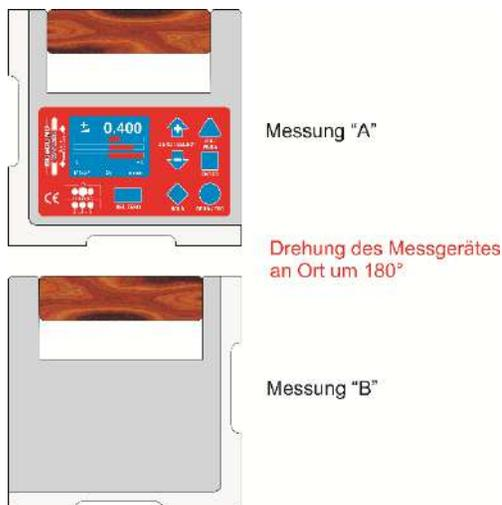
The absolute zero is automatically determined through a **reversal measurement** (two measurements in opposite directions, but from the same position). To carry out this procedure, choose a suitable surface (rigid, stable support, and as smooth and horizontal as possible) that you can place the wylerLEVEL on. Mark the position and orientation of the wylerLEVEL precisely, and then rotate it 180° in the same spot.
