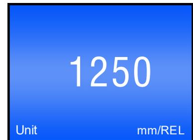
When measuring in Relative Mode, the height X is displayed as linear measure in relation to the base length entered (in **mm** or **inches**).
