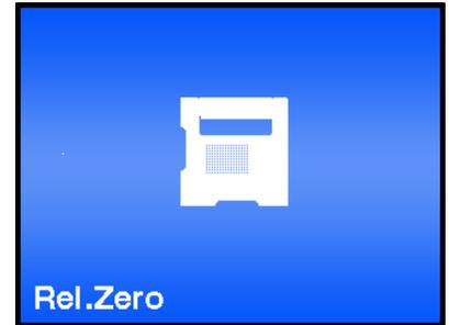
Place the wylerLEVEL in position and press the
