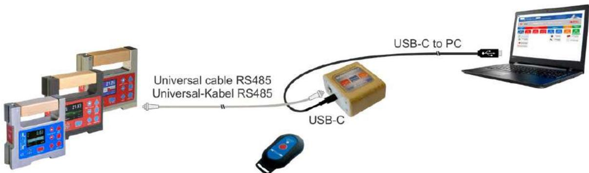
Connect wylerLEVEL / wylerCLINO to a PC using a cable connection via wylerCONNECT
