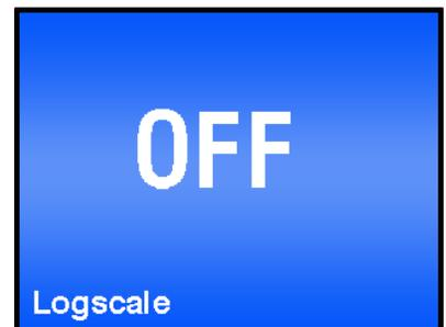
The measuring device returns to Measuring mode. When logarithmic scaling is active, the indication LOG appears under the graphic.
