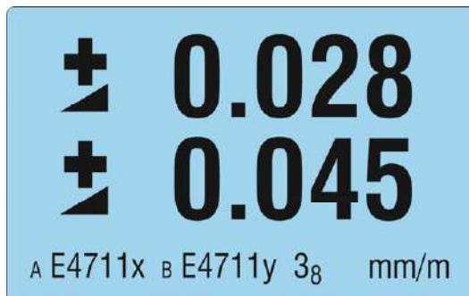
While the measuring values are continuously updated for the ZEROMATIC 2/2 (in the frequency of the parameter "measuring interval"), for the ZEROMATIC 2/1 the values after the last reversal measurement are shown.
