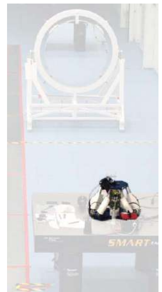
The hexapod is part of the ESA StarTiger-2 test to simulate a way to eclipse the Sun with two satellites flying in tight formation.
