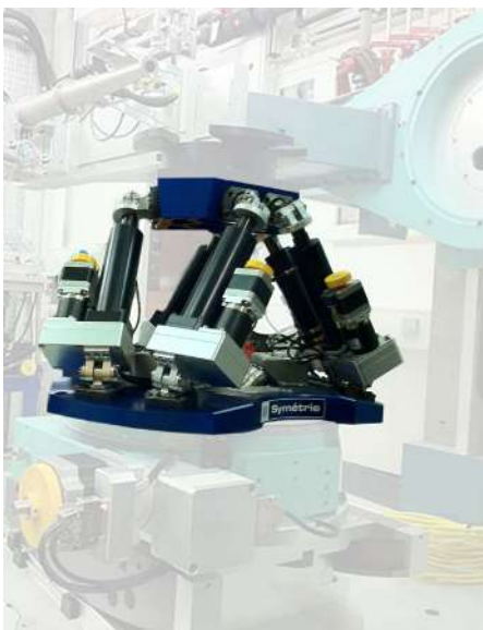
This hexapod positions a vacuum chamber containing a gas sample and offers a \pm 20^\circ angular range.
