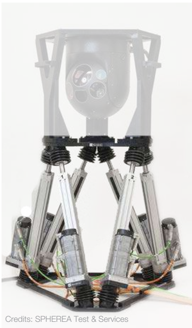
NOTUS hexapod helps to characterize and calibrate electro-optics gimbals that will be later installed on helicopters.
