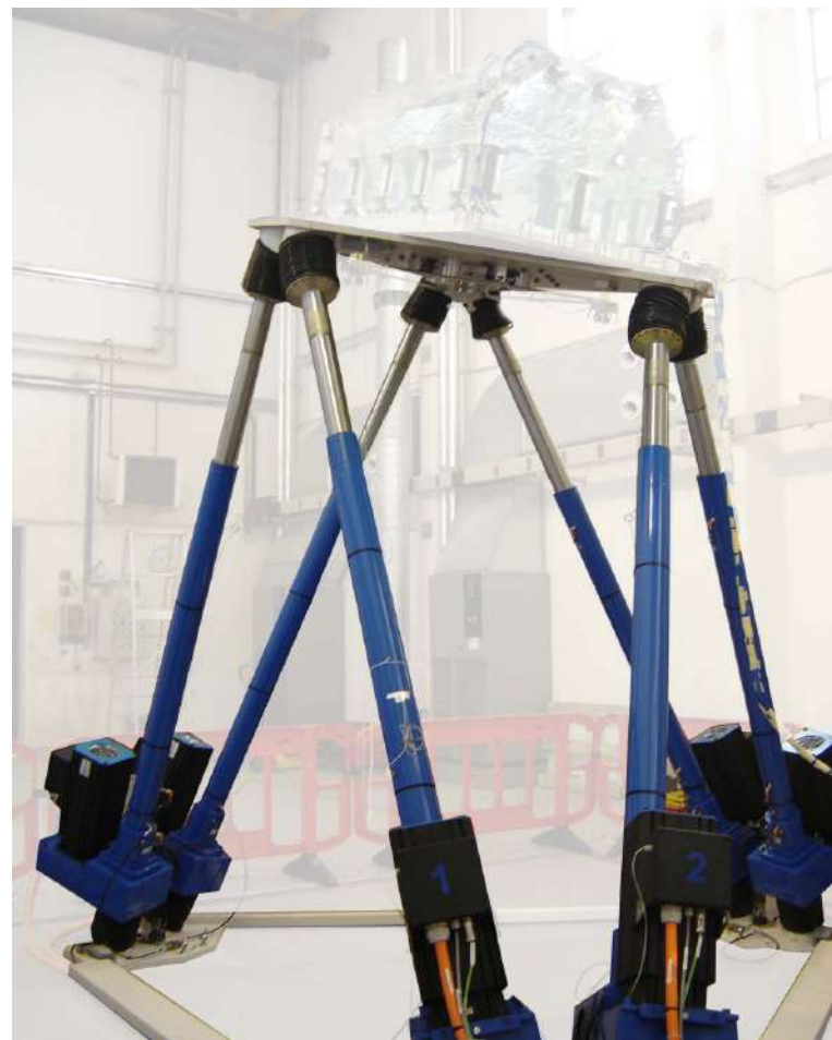
Hexapod AQUILON for sloshing tests
