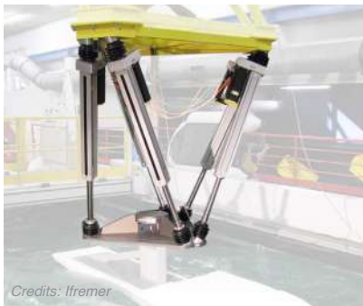
Credits: Ifremer MISTRAL hexapod orientates a ship model in a wave basin to reproduce maritime conditions and test the shipbuilding techniques.
