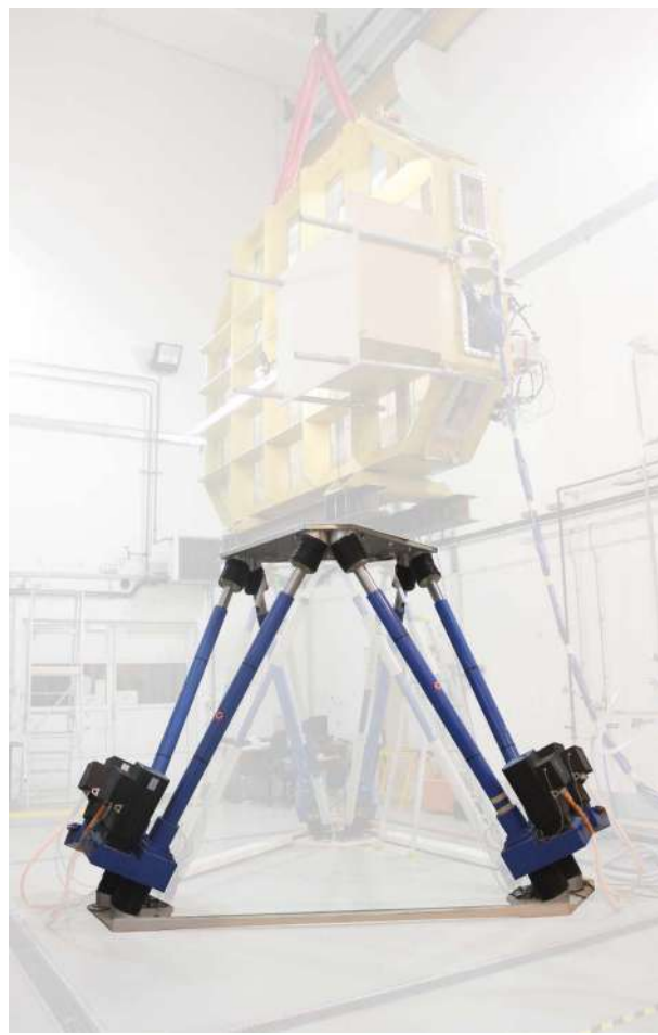
Hexapod AQUILON for sloshing tests
