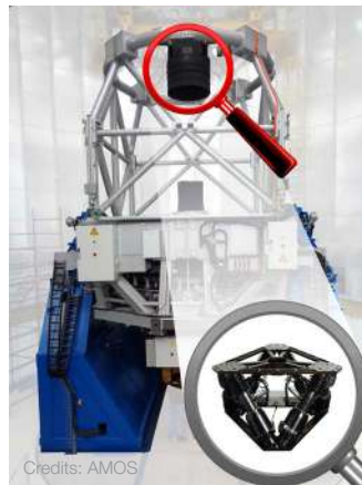
ARIES telescope is installed in Nainital in India. With a primary mirror of 3.6 m diameter, it is the largest optical centre in the country. Cross-coupling of SURES hexapod is less than 0.7 arcsec in tip-tilt during centering or focus.
