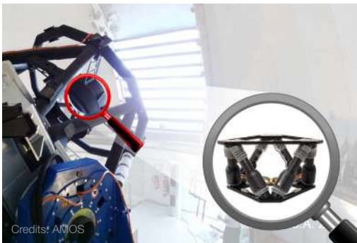
SURES hexapod positions the 450 kg secondary mirror of OAJ T250 telescope in Spain with 0.35 \mu\text{m} linear and 0.5 arcsec angular resolutions. The SURES hexapod for OAJ has a 920 mm diameter.
