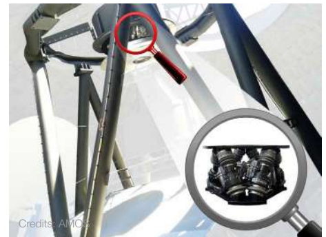
The hexapod is installed on Pan-STARRS-2 telescope at an altitude of 4267 m on Maui, Hawaii. A smaller version of SURES has been adapted as the secondary mirror is 600 mm diameter and weighs less than 110 kg.
