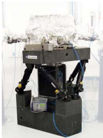
JORAN hexapod has been developed in collaboration with ESRF synchrotron to position mirrors with very high resolution.
