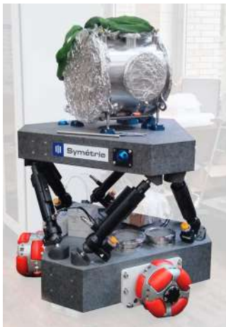
JORAN hexapod size has been adapted to the beam height of the Australian Synchrotron.
