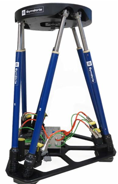
This customized hexapod with extra travel range enables the qualification of space optical instruments. Hexapod height in middle position: 1400 mm / Payload: 200 kg.
