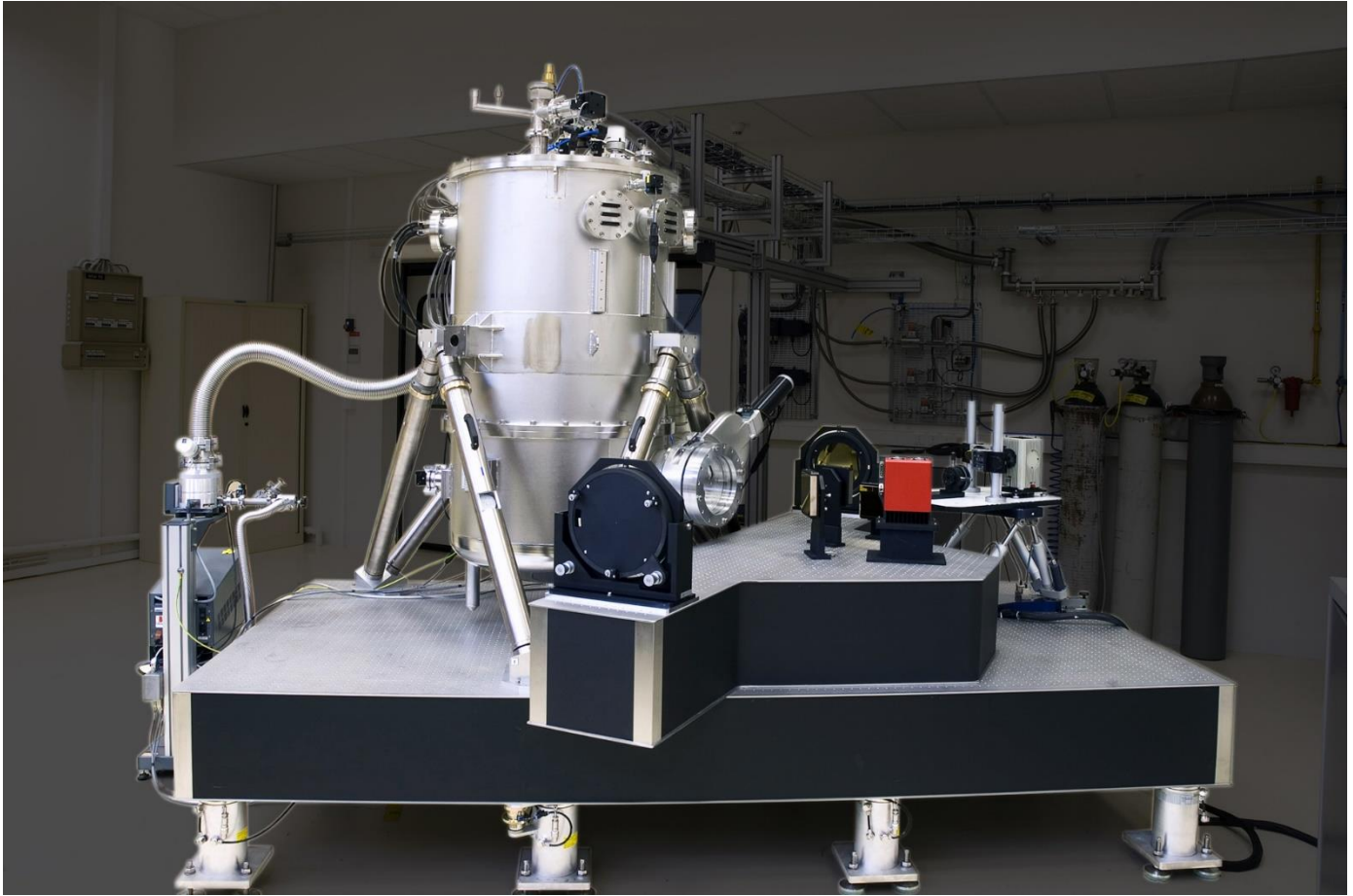
CREDITS: CEA SYMETRIE - OPTICAL TEST BENCH OF MIRIM IMAGER OF JAMES WEBB SPACE TELESCOPE
