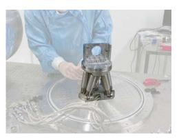
Some HV BORA hexapods are positioning the high reflectivity mirrors of a Fabry-Perot cavity in order to optimize their alignment and thereby the cavity finesse.
