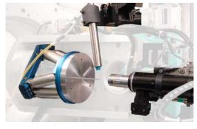
This hexapod places a sample at the centre of two large rotation stages. With this installation, hexapod mounting orientation varies between 0° and 90°. Advantages of the hexapod are: high stability, stiffness and repeatability of the sample position with respect to the rotation stages independently of their orientations.
