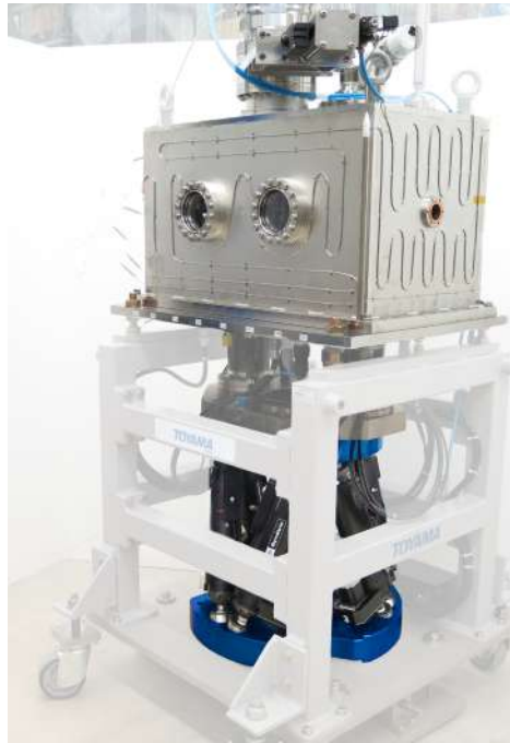
KUBAN hexapod aligns a polarimeter with high precision in a short time. This installation made by TOYAMA can be moved to be used on different beamlines at MAX IV Laboratory synchrotron.
