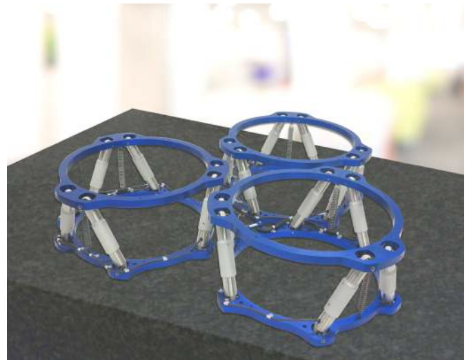
The diameter of these customized PUNA hexapods has been changed in order to maximize its central aperture (372 mm). The application is mirror alignment.
