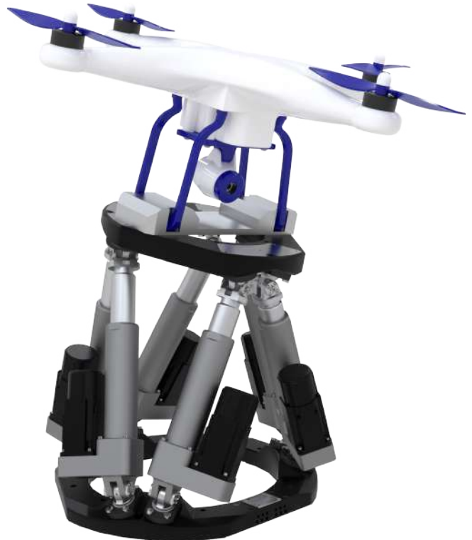
Hexapod HEGOA with a drone equipped with a camera to test the reactions of the whole during movements in flight, simulated by the hexapod.
