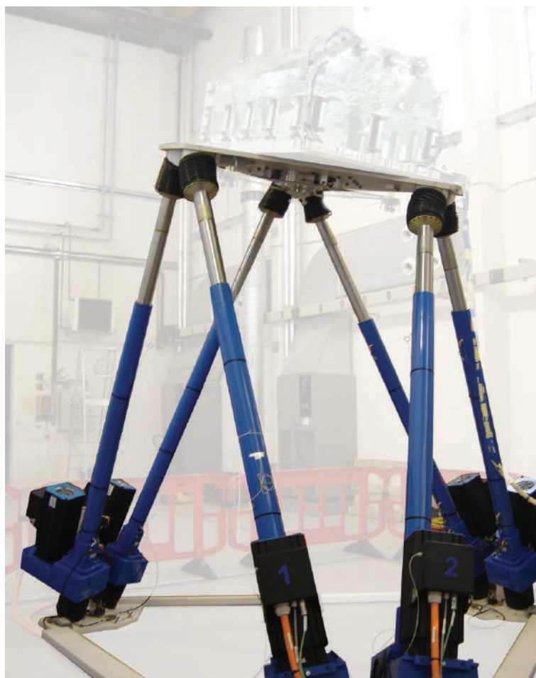
Hexapod AQUILON for sloshing tests.
