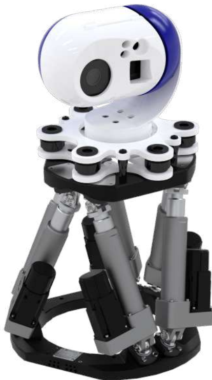
HEGOA hexapod with stabilized Giro optical component for motion compensation test.
