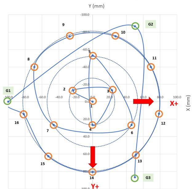
Figure 21 - Travelling pattern for cross coupling measurement on the flat mirror
