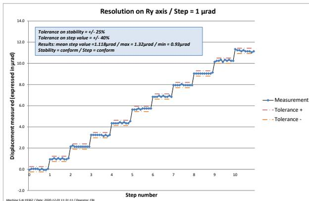
Figure 19 - Resolution around Y axis
