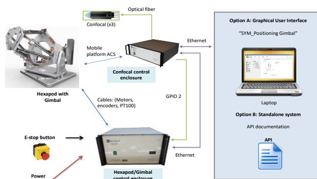
Figure 11 - Control architecture
