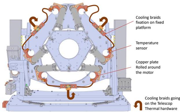
Figure 7 – Thermal braids on hexapod motors
