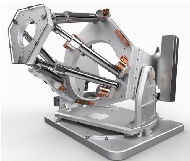
Figure 1 – Positioning system especially developed by SYMETRIE for the project (realistic CAD view)
