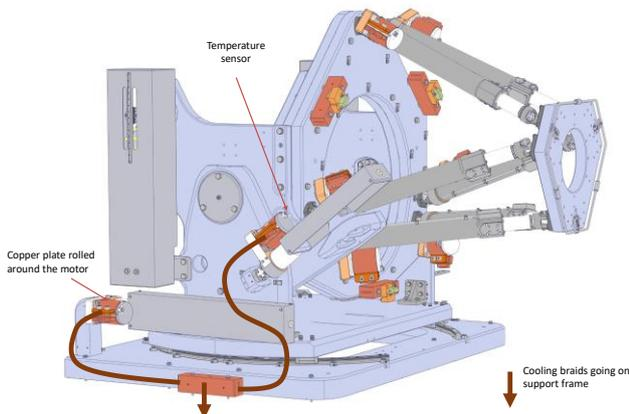
Figure 8 - Thermal braids on Gimbal motors
