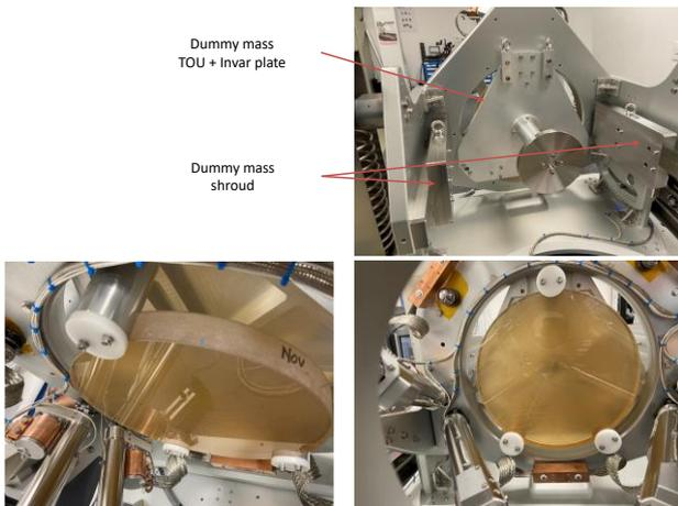
Figure 14 - Dummy load of the Unit Under Test (UUT)
