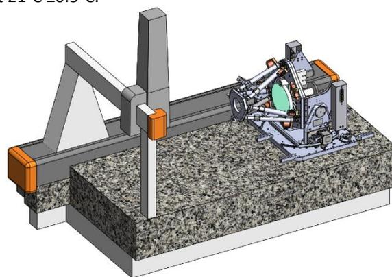
Figure 12 - Complete machine is qualified on a CMM (CAD view)
