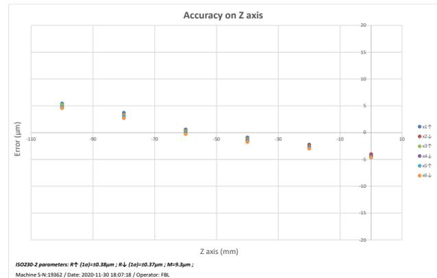
Figure 20 - Accuracy plot on Z axis
