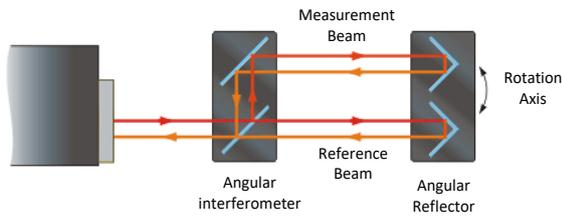
Figure 17 - Angular measurement principle with laser interferometer
