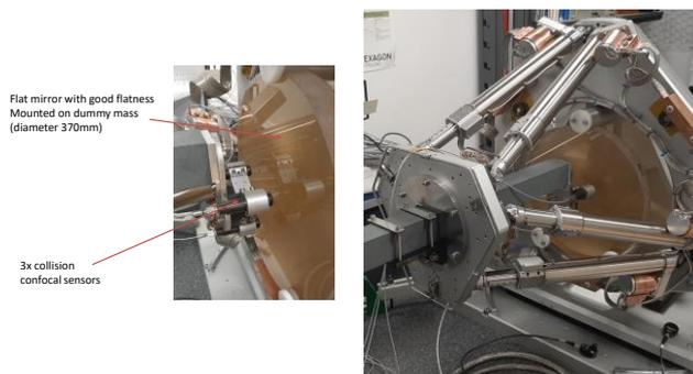
Figure 15 - Dummy detection system assembly
