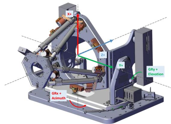
Figure 9 – Complete positioning system with the axes and dimensions
