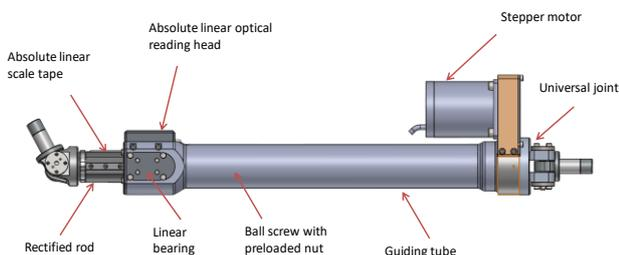
Figure 4 - Design of actuator and joints
