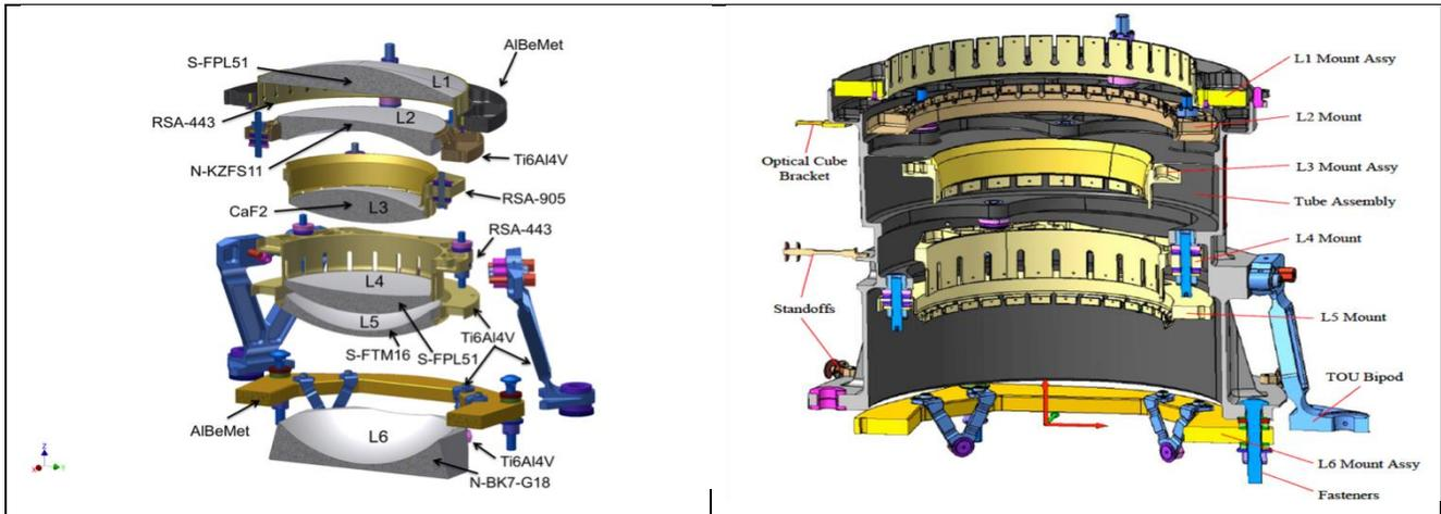
Figure 1 – *Left*: an exploded view of a PLATO’s TOU with a focus on the materials used for the glasses, their mounts, and for the interface components. *Right*: Details of the mechanical structure with subcomponents highlighted.
