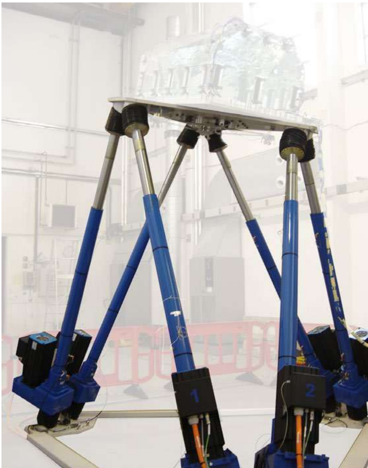
Hexapod AQUILON for sloshing tests.
