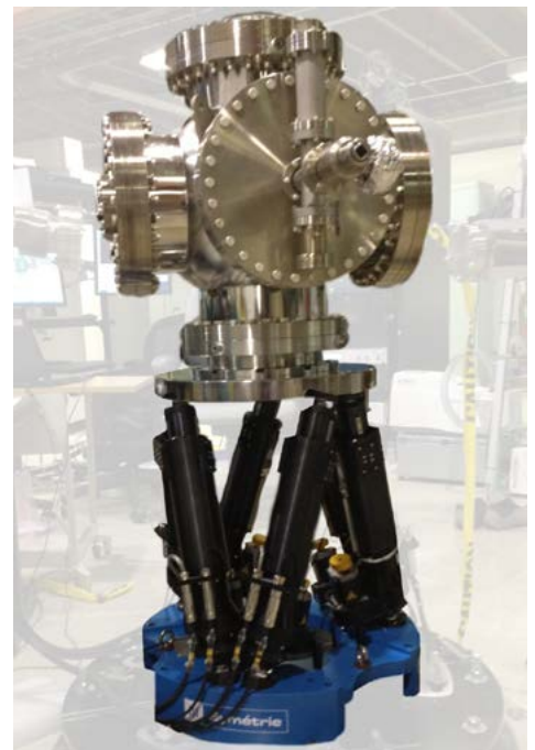
KUBAN hexapod positions a mirror inside of a vacuum chamber with high resolution. To be sure to avoid harming any part due to an unexpected over range, an inclination limit switch is installed under the hexapod mobile platform and stops the motion if the maximum roll angle is reached.
