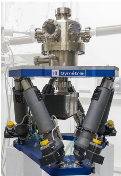
This KUBAN hexapod aligns a mirror inside a vacuum chamber on LUCIA beamline at Synchrotron SOLEIL. A high stability over time is crucial.
