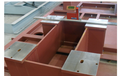
Coplanarity, flatness of surfaces
