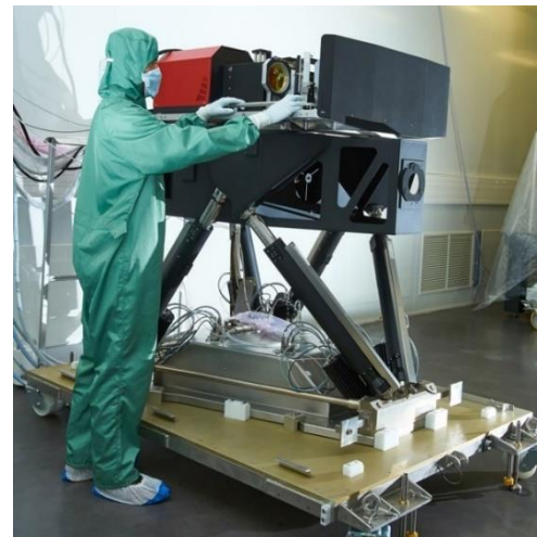
Figure 12: Setup with CMM used to determine the look-up table (on the left) / Photo of the hexapod on customer site with instrument mounted on it. Photo on the right copyright Bertin Technologies.
