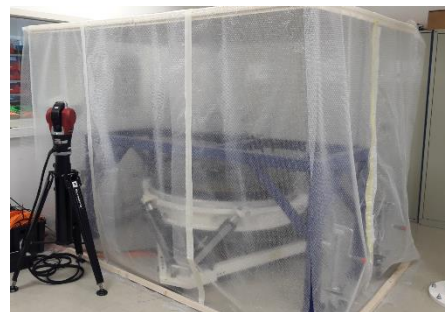
Figure 20: Setup with 6 capacitive sensors to measure positioning performances on the 6 degrees of freedom at the same time.
