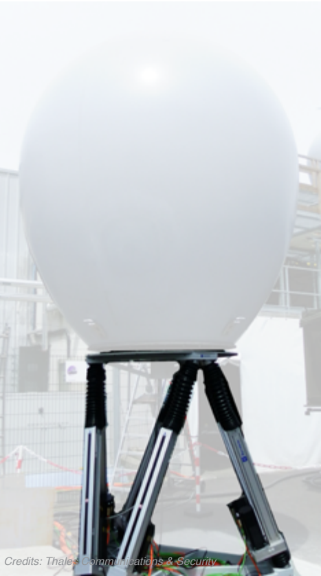
Credits: Thales Communications & Security MISTRAL hexapod reproduces ship motions to test the stabilization performances of large maritime SATCOM antennas.
