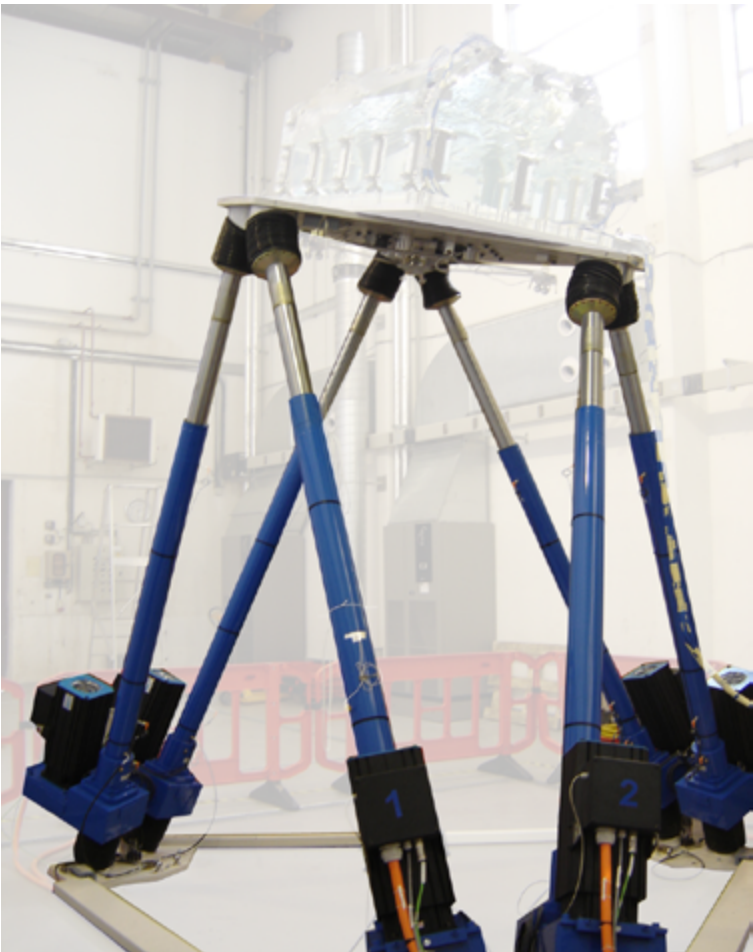
Hexapod AQUILON for sloshing tests.
