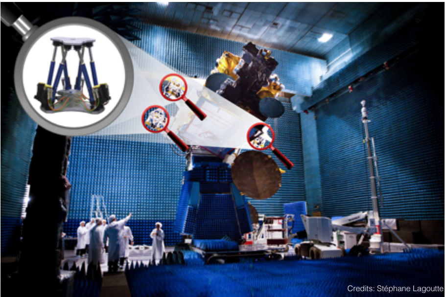
Four SIRIUS hexapods orientate the antennas of telecommunication satellite to test their performances before the launch. Thanks to the flexibility and pivot point configuration of these hexapods, this set up is adaptable to different satellite models.
