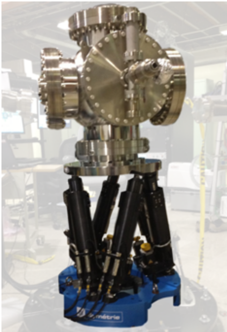
KUBAN hexapod positions a mirror inside of a vacuum chamber with high resolution. To be sure to avoid harming any part due to an unexpected over range, an inclination limit switch is installed under the hexapod mobile platform and stops the motion if the maximum roll angle is reached.
