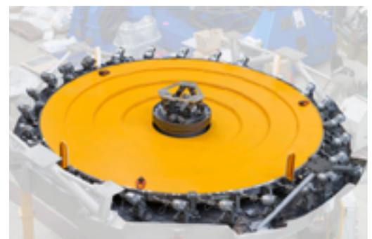
*Two identical SURES hexapods position the M2 and M3 mirrors of DAG 4m telescope in Turkey. They realign the optics in order to compensate relative displacements due to gravity and temperature change during observation. Thus they improve the imaging quality of the telescope.*
