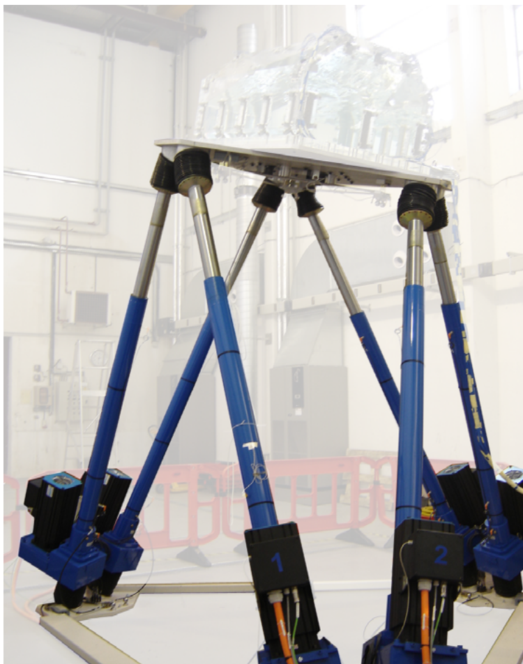
Hexapod AQUILON for sloshing tests.
