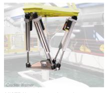
MISTRAL hexapod orientates a ship model in a wave basin to reproduce maritime conditions and test the shipbuilding techniques.
