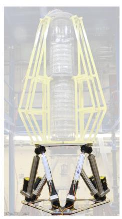
MISTRAL hexapod simulates the motion of a floating gas production unit to characterize hydrodynamic effects of swell on the chemical reactions in a gas deacidification column. These tests allow to improve performance and robustness of the processing units.
