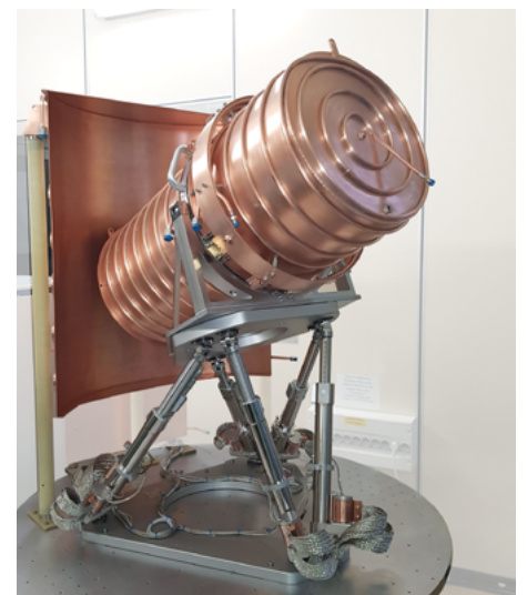
This HV ZONDA hexapod is used for the thermal vacuum tests and calibration of some of the cameras of PLATO mission at IAS.
