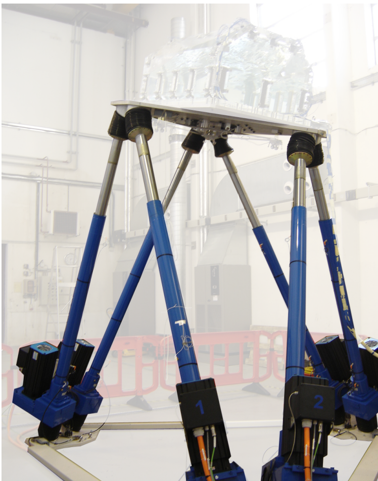
Hexapod AQUILON for sloshing tests.
