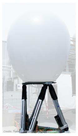
MISTRAL hexapod reproduces ship motions to test the stabilization performances of large maritime SATCOM antennas.
