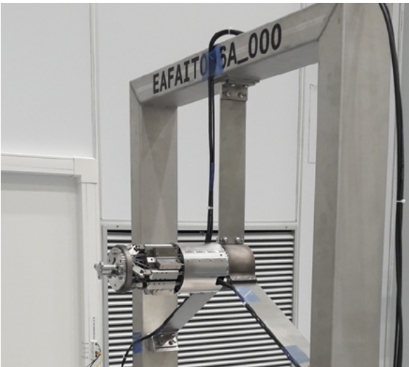
MAUKA hexapod has a very small diameter of 107 mm.
