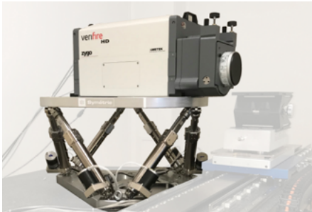
This ZONDA hexapod positions a laser interferometer (Zygo) in order to characterize the X-ray mirrors at Synchrotron SOLEIL.
