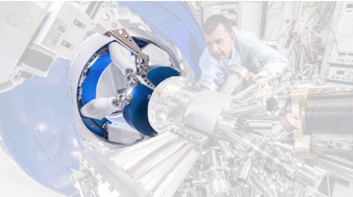
Diffraction experiment with BREVA hexapod on CEA BM32 beamline at ESRF synchrotron for the development and analysis of nanomaterials.
