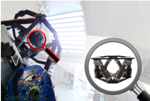
SURES hexapod positions the 450 kg secondary mirror of OAJ T250 telescope in Spain with 0.35 \mu m linear and 0.5 arcsec angular resolutions. The SURES hexapod for OAJ has a 920 mm diameter.
