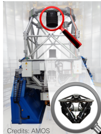
ARIES telescope is installed in Nainital in India. With a primary mirror of 3.6 m diameter, it is the largest optical centre in the country. Cross-coupling of SURES hexapod is less than 0.7 arcsec in tip-tilt during centering or focus.
