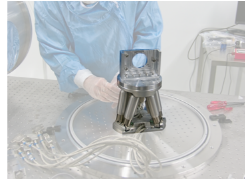
Some HV BORA hexapods are positioning the high reflectivity mirrors of a Fabry-Perot cavity in order to optimize their alignment and thereby the cavity finesse.
