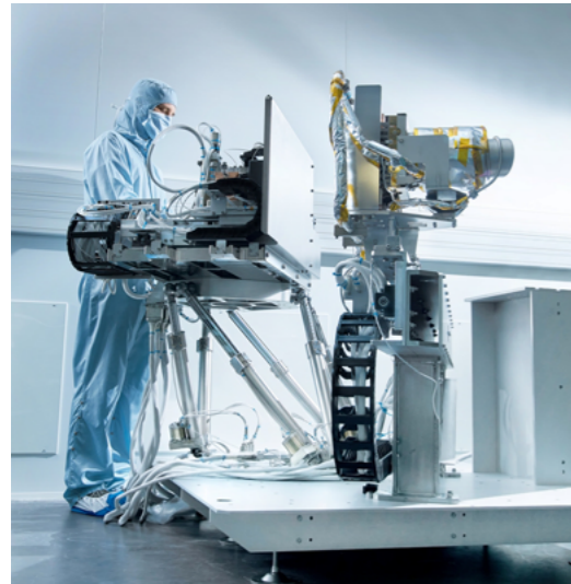
ISO5 clean room compatible hexapod to test space optical instruments for MTG (Meteosat Third Generation) satellites at BERTIN Technologies.
