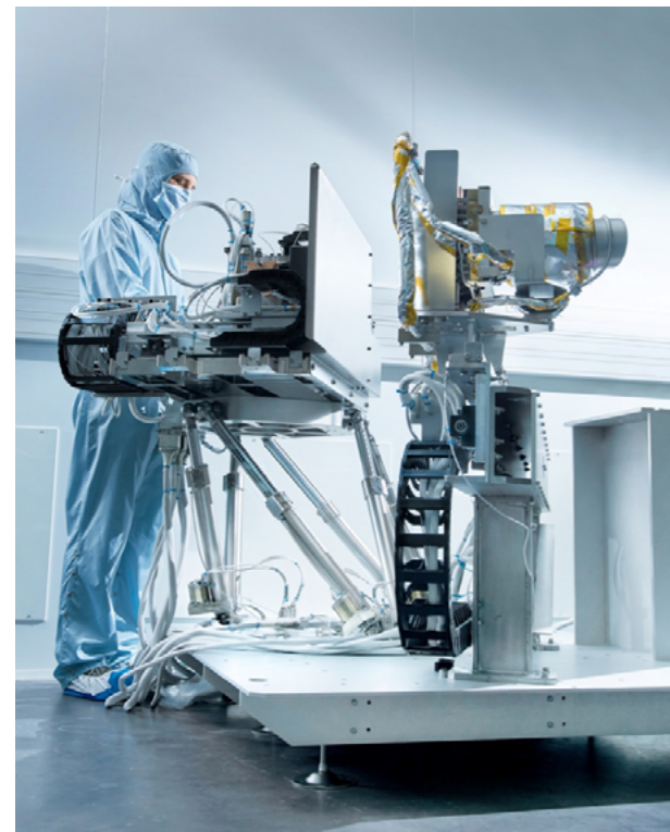
ISO5 clean room compatible hexapod to test space optical instruments for MTG (Meteosat Third Generation) satellites at BERTIN Technologies.
