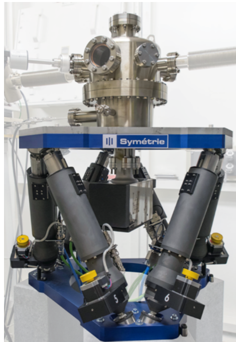
This KUBAN hexapod aligns a mirror inside a vacuum chamber on LUCIA beamline at Synchrotron SOLEIL. A high stability over time is crucial.
