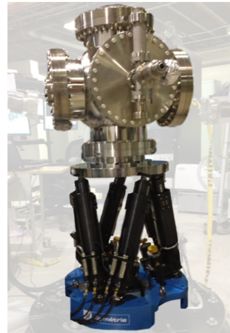
KUBAN hexapod positions a mirror inside of a vacuum chamber with high resolution. To be sure to avoid harming any part due to an unexpected over range, an inclination limit switch is installed under the hexapod mobile platform and stops the motion if the maximum roll angle is reached.
