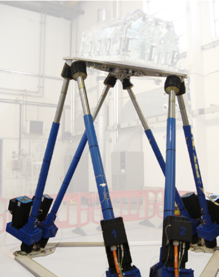
Hexapod AQUILON for sloshing tests.
