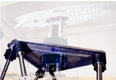
Credits: IGN-ENSAM The surfers can practice various wave situations played by our Simusurf hexapod and improve their gestures through practice and analysis by recording their movements with additional sensors. Simusurf hexapod can be used as a discovery and learning tool for the casual surfer or as a performance and training tool for the professional surfer.
