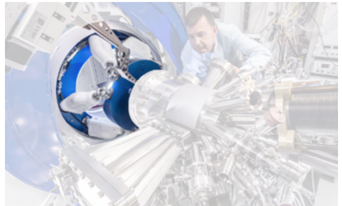
Diffractometer with BREVA hexapod on CEA BM32 beamline at ESRF synchrotron for the development and analysis of nanomaterials.
